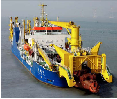
Figure 15: Tian Jing Hao, Cutter-Suction Dredge (Annex 858)
